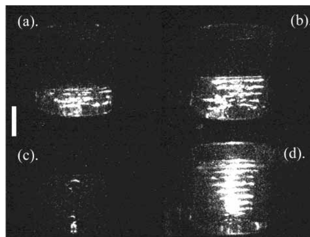
Figure 10. Frames showing the light emission from a cylindrical double-walled cell (5.8 cm internal diameter, 8.5 cm external diameter, and height 12 cm) recorded from the side. In all cases, the driving voltage was maintained at 130 V. The cell contained an aqueous solution identical to that reported in the legend of Figure 3. The cell was jacketed at 25 °C under aerobic conditions. The applied frequency was 104 kHz for all frames. In frame a, the solution height was 28 mm; frame b, 42 mm; frame c, 61 mm; and frame d, 80 mm. The scale bar represents 28 mm.
